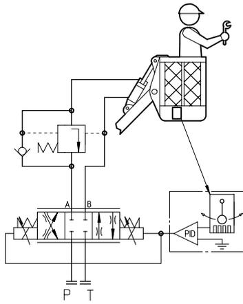
This typical application provides automatic levelling of platform using a proportional valve controlled by a specific electronics that includes levelling gauge plus electronic driver in closed loop. The whole electrohydraulic system is a compact module directly applied on board.
