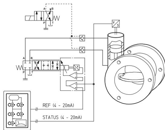
Remote control of process valves is easily achieved by electrohydraulic systems: a set reference signal ranging from 4 to 20 mA defines the opening position and therefore the valve regulations in closed loop, with resident monitor output for possible security controls. The integral electronic driver may be directly controlled through 4-20 mA signal generated by the remote process computer. Safety block is provided by check valves piloted by an on-off solenoid valve.
