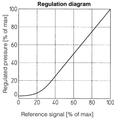
How the valve-regulated pressure varies according to the reference signal
