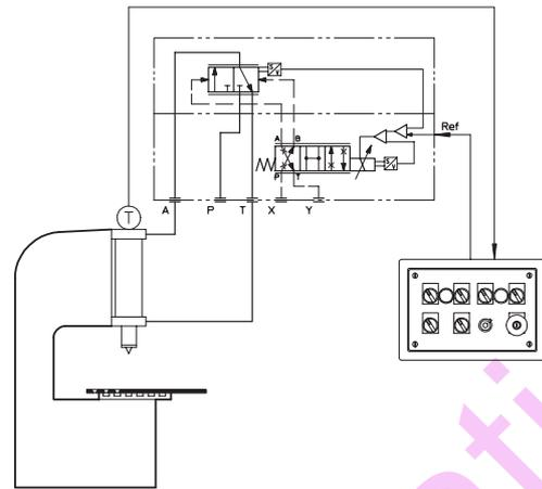
The scheme shows a regenerative circuit using a proportional cartridge valve with integral electronics, set to drive a high frequency punching-press. High performances are achieved by a closed loop control through a stroke transducer on the punching cylinder.
