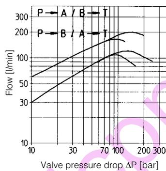
Regulated flow vs. functional  $\Delta p$  at max reference electric signal
