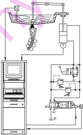
In steel work application, robust electrohydraulic units are specifically designed to assure reliability and performances. The example shows a specific electrohydraulic system to regulate the level of ible steel, including a proportional valve with integral electronics, a safety manual override equipment, a hydraulic servocylinder with potentiometric transducer and an integral manifold enclosing the control valves: the whole preset and ready to work.
