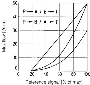
How the valve-regulated flow varies according to the electric reference signal
