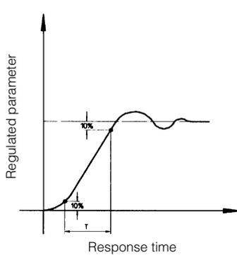
The time lag required for the valve to reach the requested hydraulic output following a step change in the reference signal (usually 0÷100%). Response time is measured in millisecond [ms] and is an easy parameter to evaluate the dynamics of the valve.
