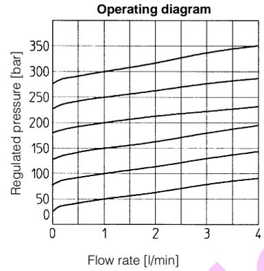
How the valve-regulated pressure varies according to the flow passing through
