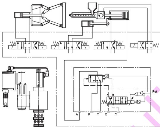
In presses for plastic materials a proportional throttle cartridge controls the three main functions, i. e. injection speed, pressure profile and mold filling counterpressure. The electronic control is performed by a proportional valve with integral electronics and with integral position transducer which closes the loop on the main poppet for precision settings and high dynamics.
