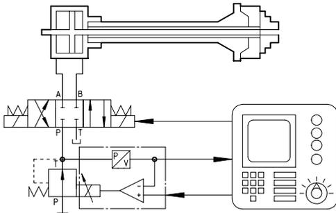
The automatic control of clamping forces is necessarily required on clamping mandrels for deep boring machining, to avoid damages to expensive tools. The controlling signal is processed by a CNC system and the proportional valve has integral pressure transducer plus closed loop electronics.
