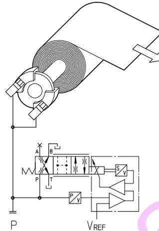
The control of pulling force in a textile warping machine is achieved by a proportional system that regulates the brake action. The valve has integral electronics able to control braking pressure in closed loop through feedback signal from the pressure transducer; unlike conventional pressure control this system features fine regulation starting from null pressure.
